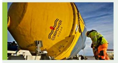
**Corpower** deployed its ½ scale C3 wave energy converter in January 2018. The device has being exposed to real-life sea conditions, following rigorous on-land test program. Testing will allow the demonstration and refinement of low-cost maintenance and inspection operations.
