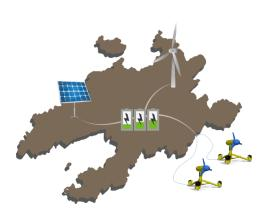
Two tidal turbines of 500 kW each, one wind turbine of 900 kW, 500 kW of innovative solar panels solutions and an energy storage (Li-Ion) of 2 MWh.
