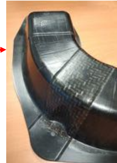
Final formed component after QSP
