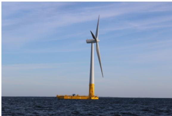
**Figure:** FLOATGEN, the prototype floating offshore wind turbine, used as a reference in this thesis. Source: <https://sem-rev.ec-nantes.fr/eolienne-flottante-floatgen/> (visited on 18/02/2019 at 17:19)
