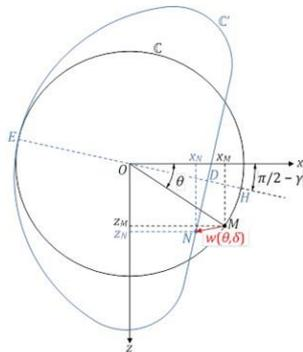
*Deformation mechanism of a tube section*
